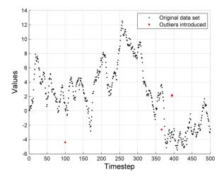
Figure 1: Synthetic data set simulated using an ARIMAX(3, 1, 1, 3) with the four outliers drawn from ARIMAX(2, 0, 1, 3) depicted on the graph
