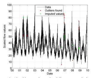
Figure 6: Algorithm result on the daily aggregated electric load data set using an ARIMAX (5, 1, 3, 3) and temperature as exogenous inputs
