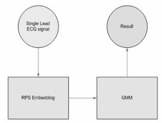
Figure 1: Block diagram describing GMM/KLT approach
